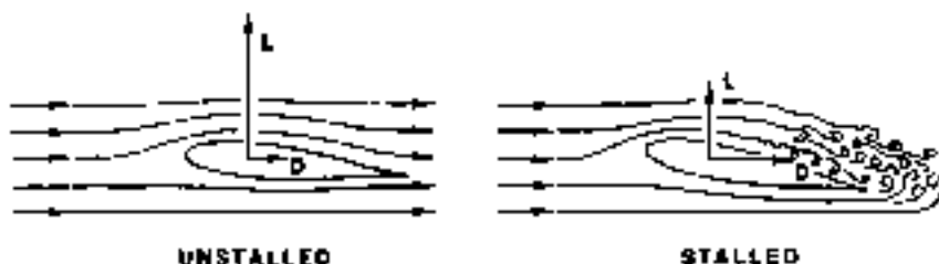
Wing or rotor blade unstalled and stalled.
