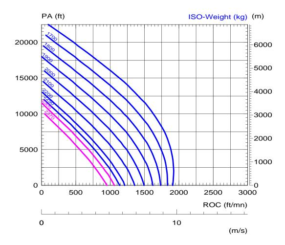
Note: Approved performance, as long as the engine meets the power check criteria, as defined in the Flight Manual for a clean standard aircraft equipped with the optional Low landing gear (see page 38).
