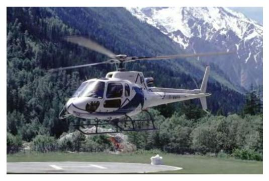
The AS350 B3 is "the high performance" version of the single engine ECUREUIL range, beating every other single engine helicopter in its category. It fulfils the FAR 27 regulation for VFR operation by day and night 1. It offers a Maximum Internal Gross Weight of 2,370 kg / 5,225 lb 2 and a Maximum all-up weight of 2,800 kg / 6,172 lb in external load configuration. This makes the helicopter perfectly suited for:
