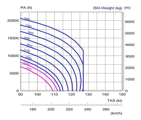
Note: Typical performance with clean baseline aircraft equipped with the optional Low landing gear (see page 38).
