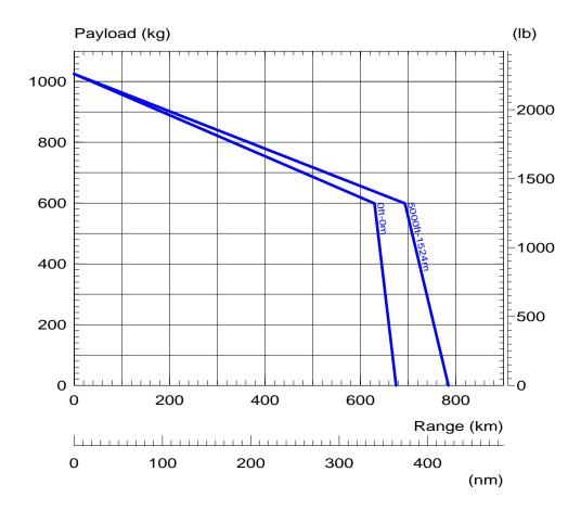
Note: Typical mission without reserve, with clean aircraft equipped with the optional Kit to Increase Internal Gross Weight to 2,370 kg (5,225 lb), with the standard High landing gear (see page 38) and new engine.
