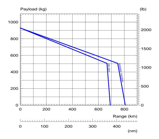
Note: Typical mission without reserve, with clean aircraft equipped with the optional Low landing gear (see page 38) and new engine.
