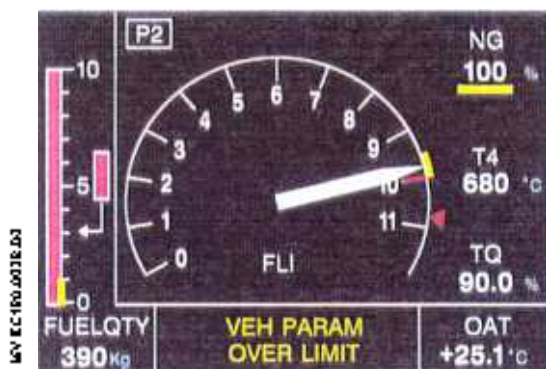
Figure 7 - 7 : FLI page (Values given as an example) fuel gauge with auxiliary tank installed (optional)
