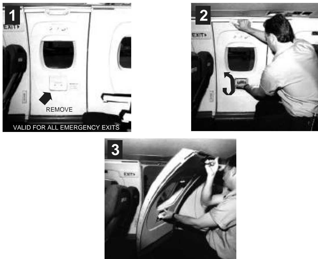
Figure 1-28. Emergency Exit Operation
