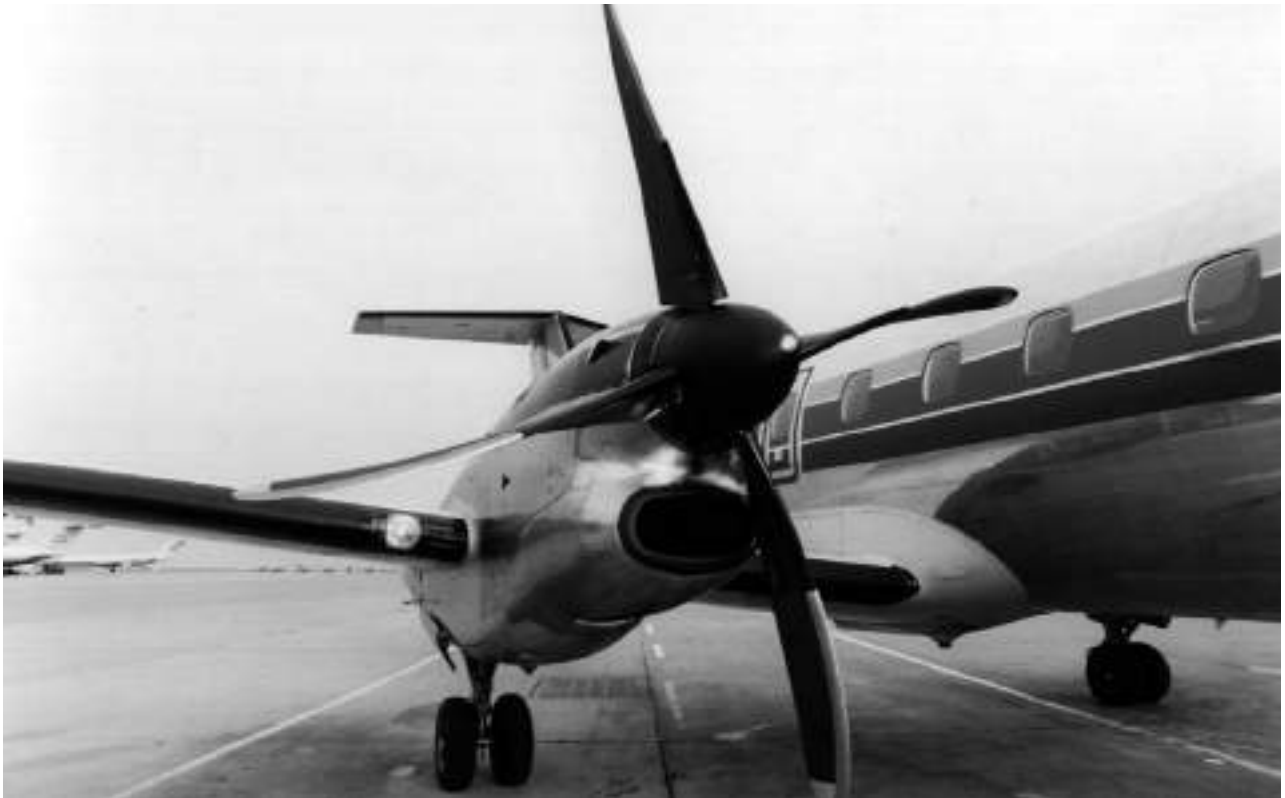
Figure 7-20. Hamilton Standard 14RF-9 “Commuter” Propeller
