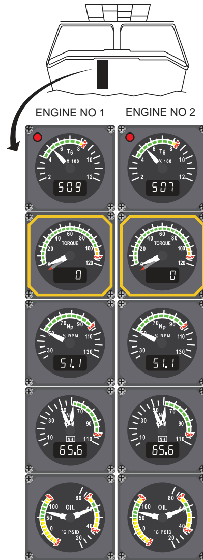
Figure 7-16. Engine Instrument Location
