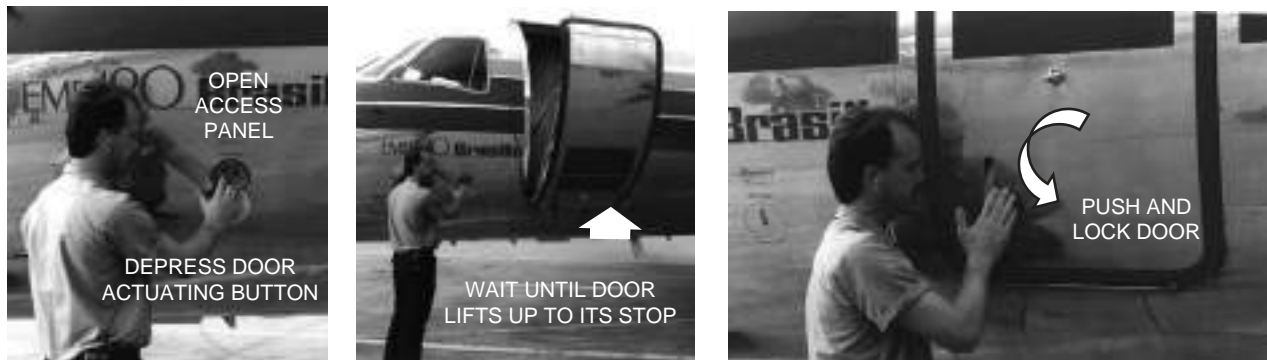
Figure 1-21. Forward Entry Door Operation
