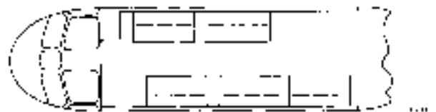
Figure 2-54. Utility Troop Seats
