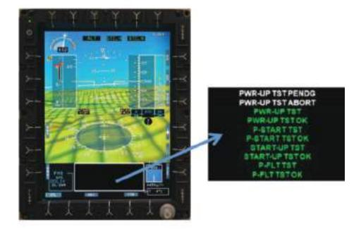
H175 benefits from all technical capacities and features to detect any symptom encountered during the flight thanks to Helionix. To facilitate maintenance operations, the new powerful Maintenance Ground Segment allows operators a fast, easy and guided analysis, and therefore an improved anticipation and reactivity on maintenance.
