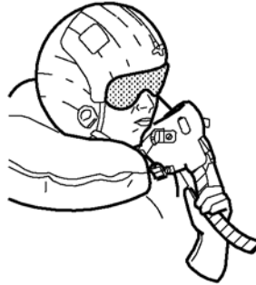
Remove oxygen mask. Oxygen mask/hose assembly may be disconnected from seat kit and discarded, if desired.
