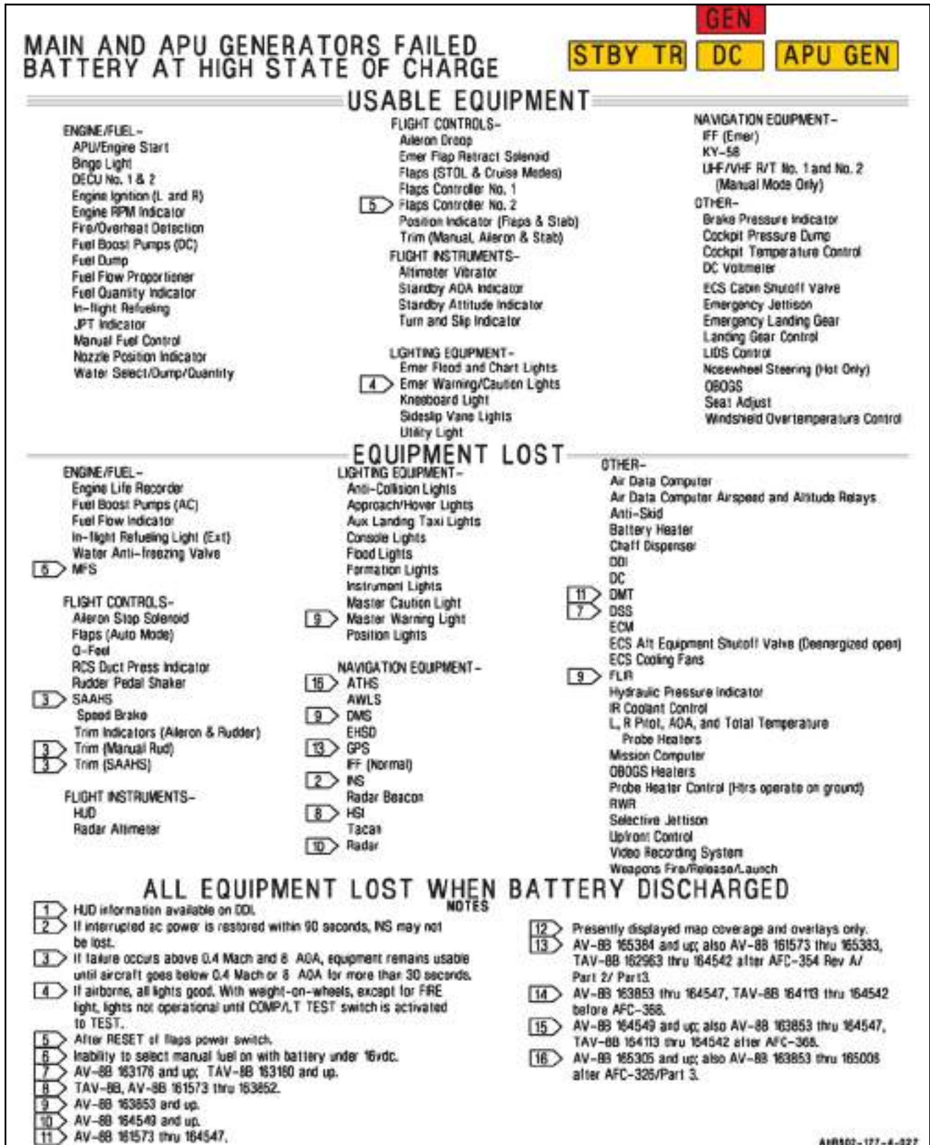
Figure 15-3. Emergency Power Distribution (Sheet 4)
