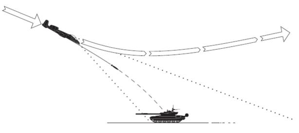
CCIP: Continuously Computed Impact Point CCPI: Calcul Continu du Point d'Impact
