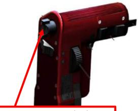
**Target Designator Caret (TDC) Switch** DEPRESSED = Radar Lock
