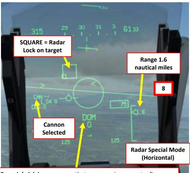
**DOM (Domain) Advisory** means that you are in range to fire your MAGIC II missiles when you are in GUN mode. DOM caution will disappear when you are closer than 1200 m from radar-locked target.
