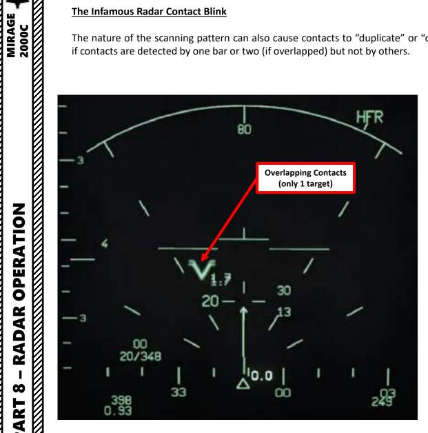
Note: V symbols just tell you the bar at which the target was detected, NOT the target's relative altitude to you.
