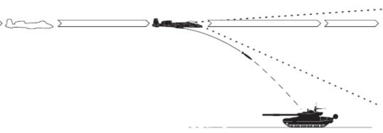
**CCRP:** Continuously Computed Release Point *CCPL:* Calcul Continu du Point de Largage
