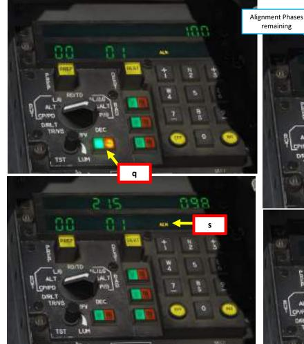
Seconds remaining Percentage of TOTAL for current Alignment Progress alignment phase remaining
