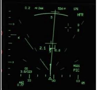
RADAR IN STT (Single Target Track)/PIC MODE One target locked Only locked target is visible, ranged and scanned 108
