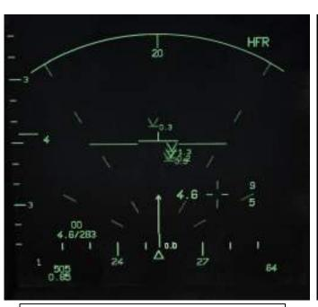
RADAR IN RWS (Range While Search) MODE No target locked All targets visible, ranged and scanned
