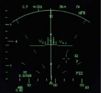
RADAR IN TWS (Track While Scan)/PID MODE One target locked All targets visible, ranged and scanned
