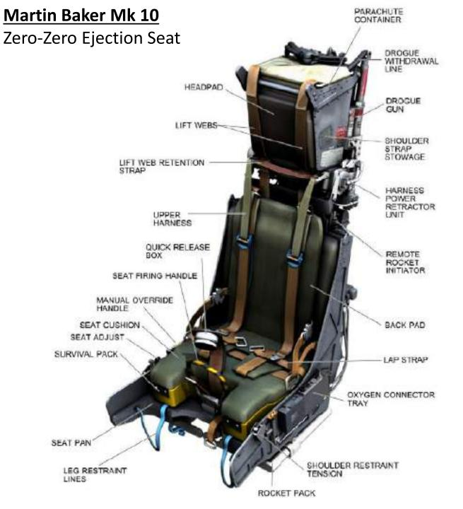
A zero-zero ejection seat is designed to safely extract upward and land its occupant from a grounded stationary position (i.e., **zero** altitude and **zero** airspeed), specifically from aircraft cockpits. The zero-zero capability was developed to help aircrews upward from unrecoverable escape emergencies during low-altitude and/or low-speed flight, as well as ground mishaps. Before this capability, ejections could only be performed above minimum altitudes and airspeeds.
