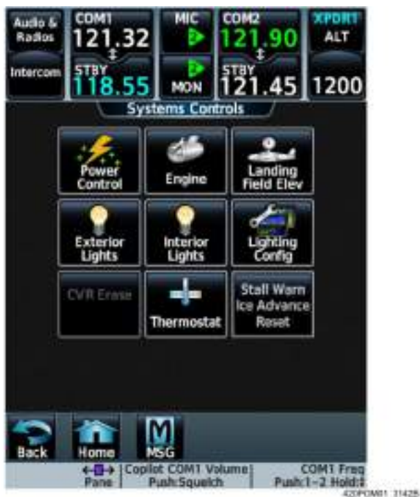
Figure 1-94. Systems Controls Page
