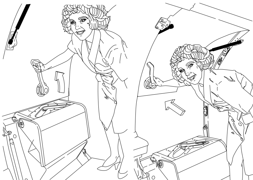
LEFT FORWARD EMERGENCY EXIT OPERATION Figure 1-9
