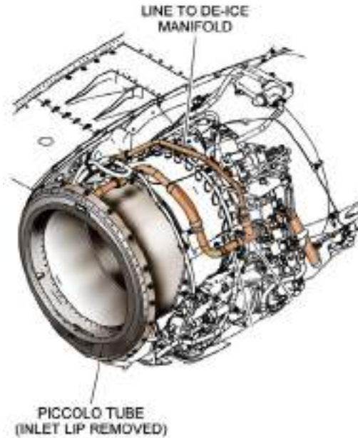
Figure 67. Engine Inlet Anti-Ice
