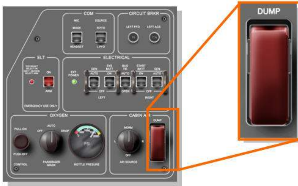
Figure 136. Cabin Dump Switch
