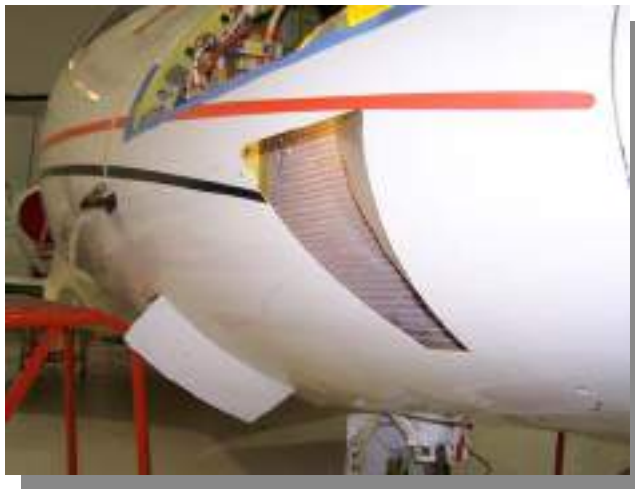
Figure 133. Condenser Inlet and Exhaust Doors
