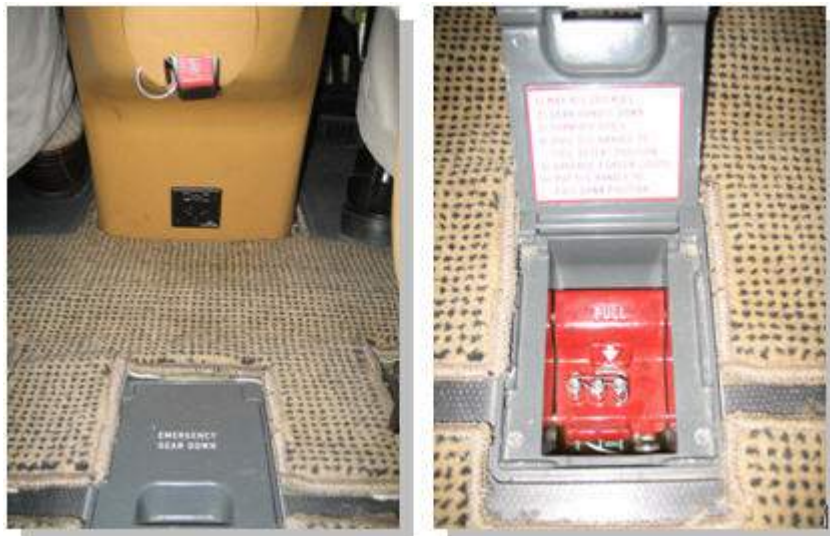
Figure 39. Emergency Gear Release Handle Location
