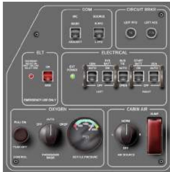
Figure 16. Left (Essential) Switch Panel
