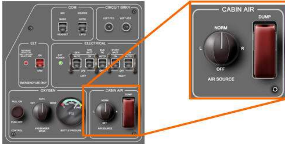
Figure 120. Cabin Air Sub Panel
