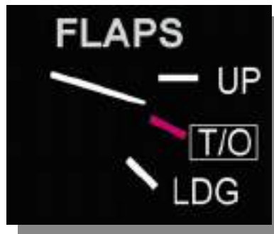
Figure 32. In Transit to T/O Position
