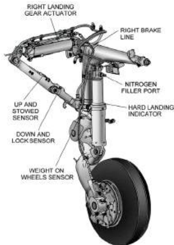
Figure 41. Main Landing Gear
