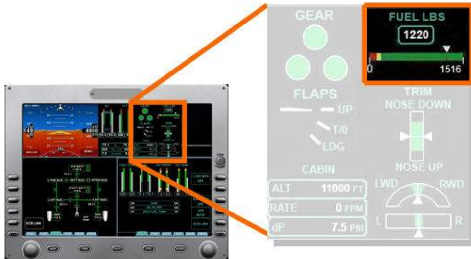
Figure 252. Fuel Quantity Display
