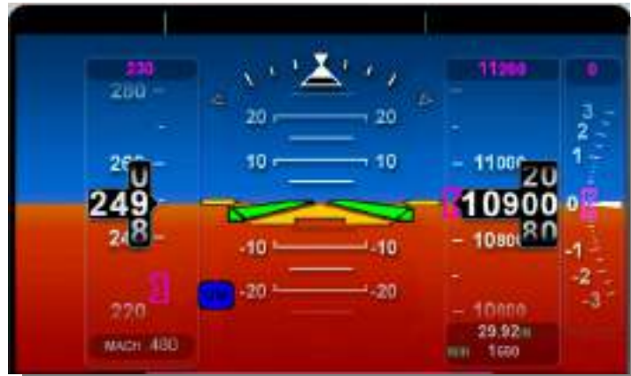
Figure 197. Outer Marker Display on PFD
