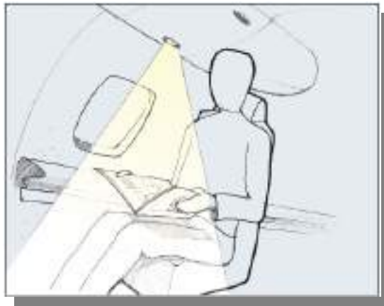
Figure 156. Cabin Reading Lights
