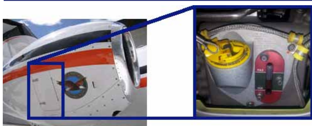
Figure 7-27. Engine Oil Sight Glass
