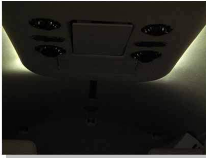
Figure 10-7. Overhead Cabin Wash Lighting
