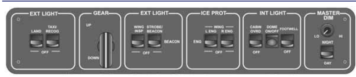
Figure 10-1. Center Switch Panel
