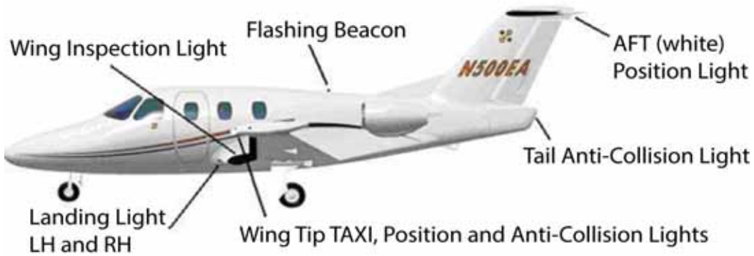
Figure 11-2. Exterior Lighting - Left Side View
