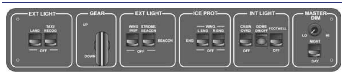
Figure 1-4. Center Switch Panel
