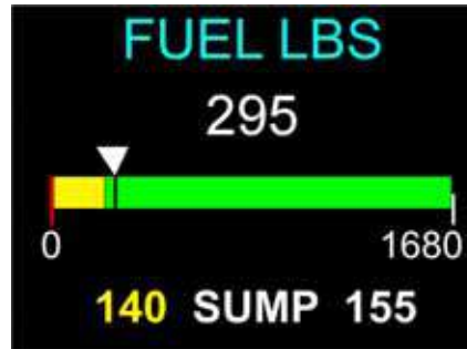
Figure 6-4. Sump Tank Quantity Display
