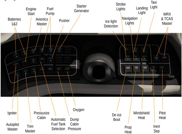
**To start the aircraft**, use the fuel tank selector on the pedestal to select the fuel tank with the larger amount of fuel. Switch on the batteries and avionics with "Batt1", "Batt2" and "Avionics".
