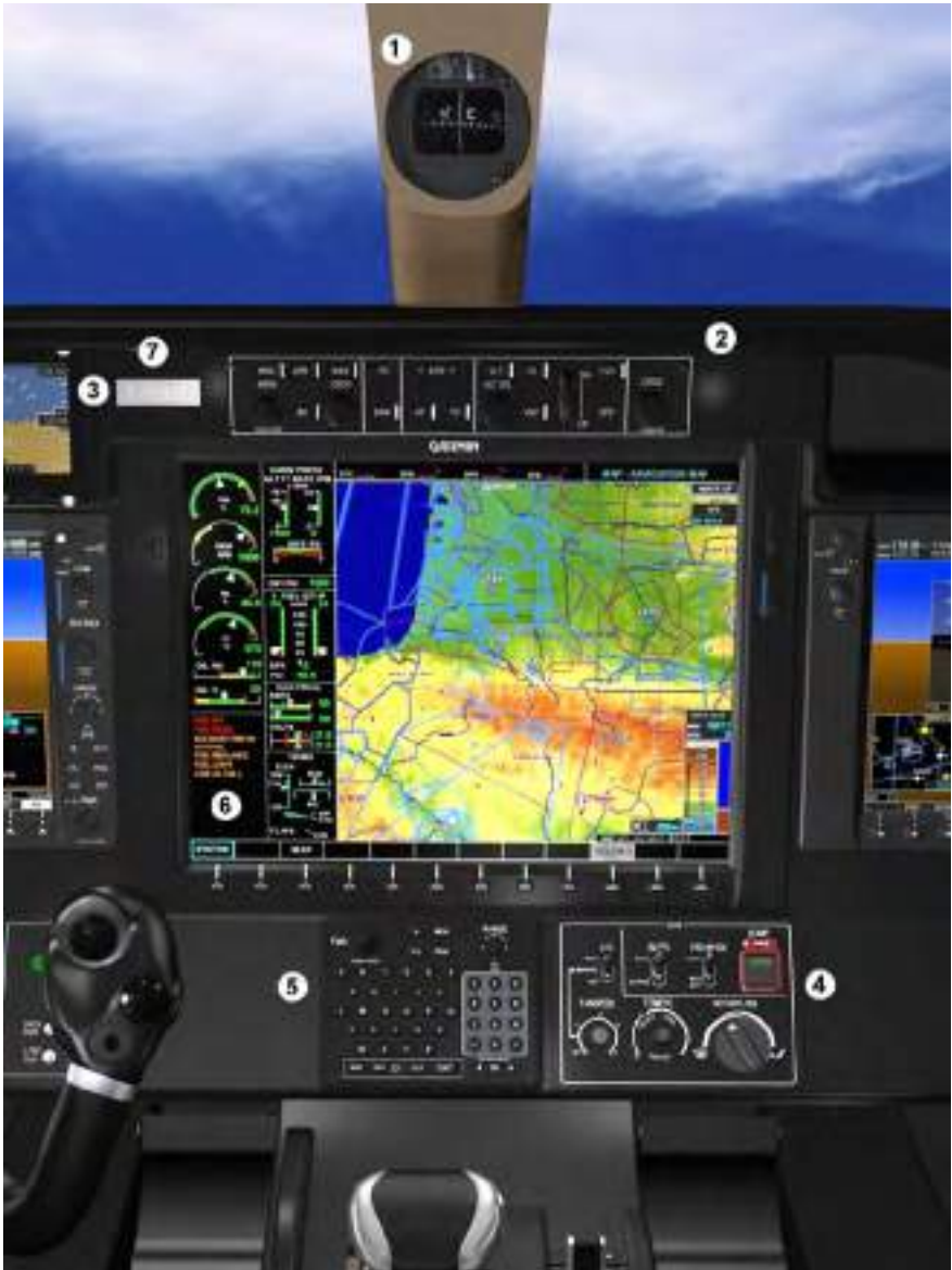
Figure 7.3.4 (2/2) - Central instrument panel (Typical arrangement) - Pre-MOD70-0529-21
