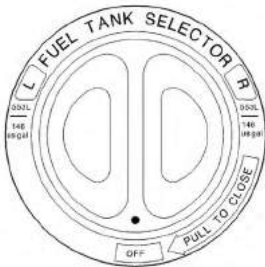
Figure 7.7.2 - Manual selector of fuel tanks
