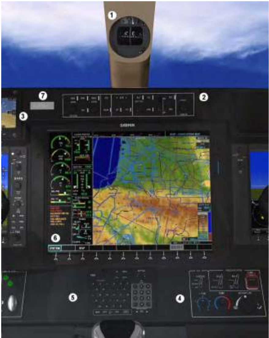
Figure 7.3.4A (2/2) - Central instrument panel (Typical arrangement) - Post-MOD70-0529-21
