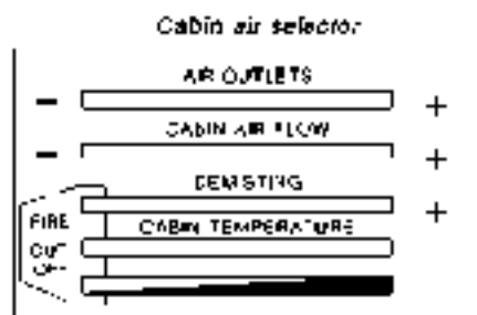
Figure 7 18 - DEMISTING, AIR REGULATION, VENTILATION, CUT-OFF SYSTEM
