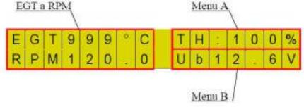
In the space for RPM and EGT indication, the display will show only physical engine speed and exhaust gas temperature. All other parameters will be displayed in Menu A or Menu B.
